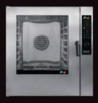
N08EMDVH 1.000x877x1.112 mm 692x450x680 mm 8 – 40 x 60 80 mm 152 Kg 400 ~ 3N 15,4 KW
